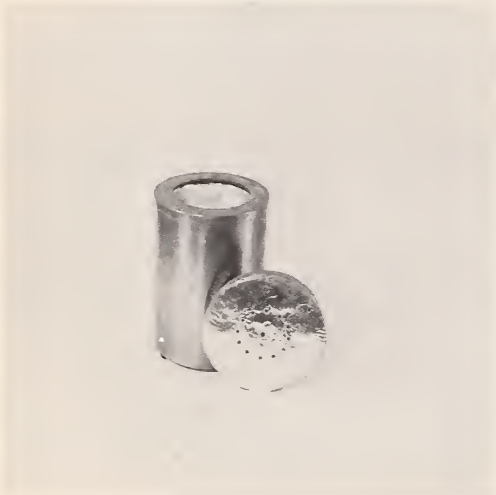
Figure 1.--Calorimeter used to determine lethal temperatures for southern pine needles.
