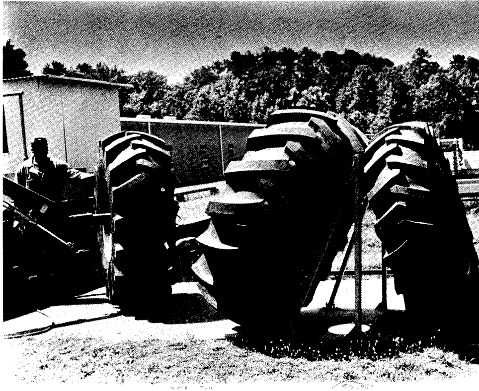
Figure 1.-Skidder tires used in load deflection tests (18.4-34 on left, 30.5L-32 in center, 24.5-32 on right).
