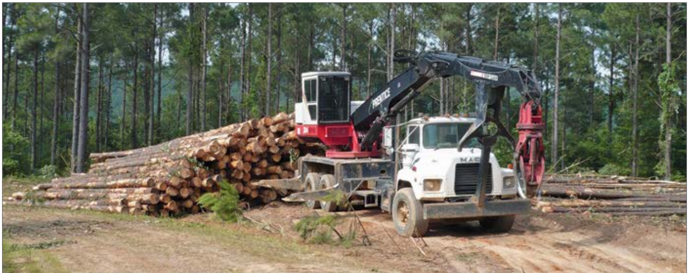
Truck mounted knuckleboom loader merchandizing loblolly pine on logging deck.
