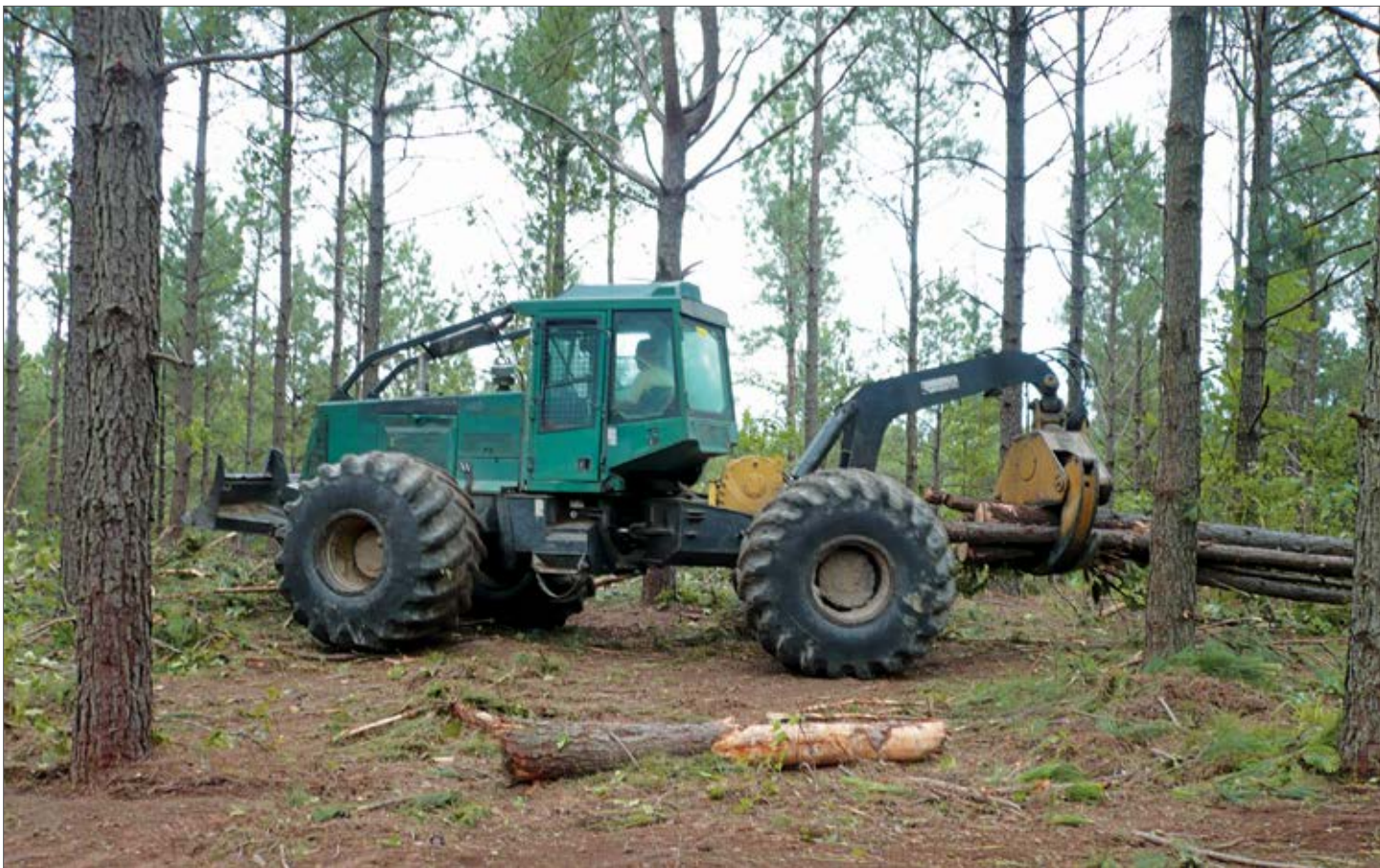
Grapple skidder pulling felled loblolly pine to logging deck.
