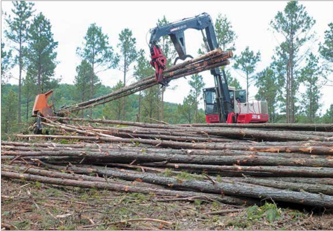
Knuckleboom loader with pull-through delimber merchandizing loblolly pine.
