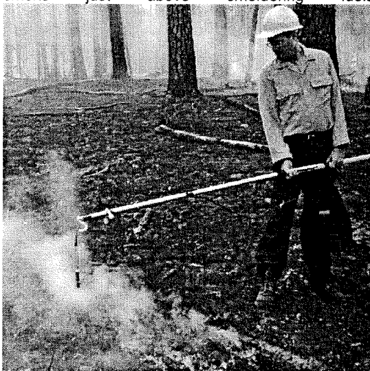
Figure 2. Sampling the temperature and relative humidity of smoke on 18 March 2002 at a prescribed burn site located at the Hitchiti Experimental Forest in central Georgia.
