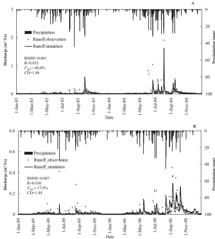
FIGURE 3. Precipitation and Annual MIKE SHE Model at Daily Time Scale Calibration (A) and Validation (B) Showing RMSE (root mean standard error),  $R$  (coefficient of correlation between measured and simulated daily streamflow),  $F_{Bal}$  (simulating errors for average streamflows), and CD (coefficient of determination).
