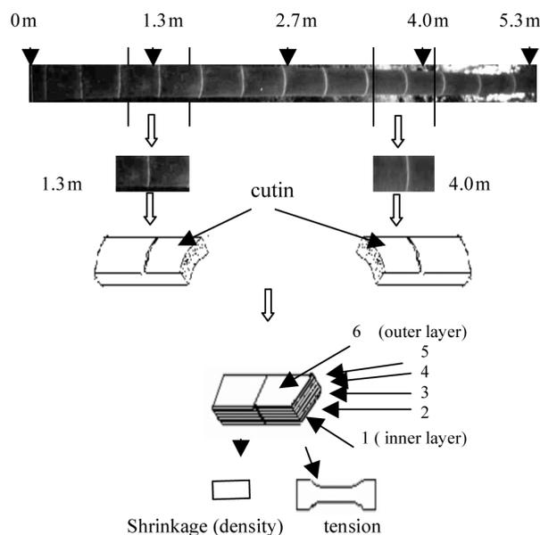
**Figure 1** Sampling sequence for the moso bamboo specimens
