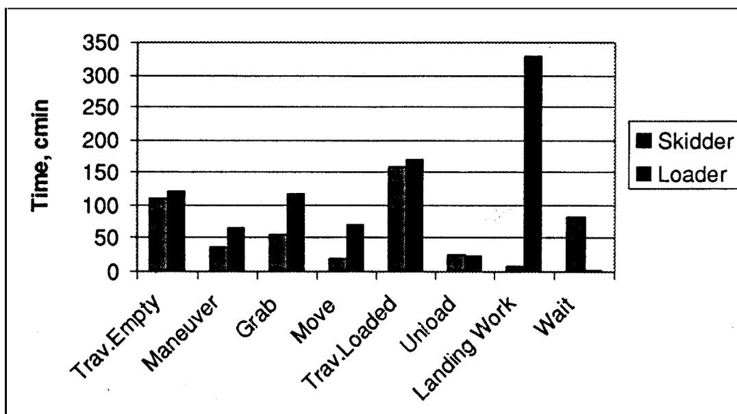
Figure 1. Time element breakdowns for the skidder and the loader.
