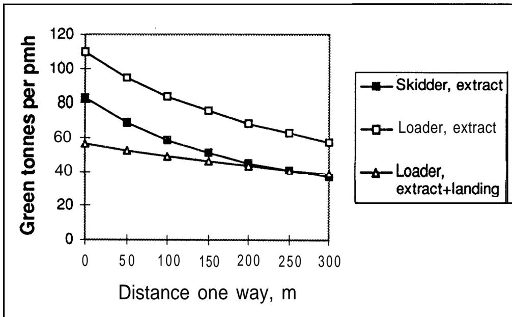
Figure 2. Productivity as a function of extraction distance.
