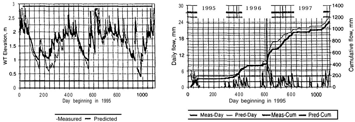
Fig. 1. Measured and predicted water table elevations (left plot) and daily and cumulative daily drainage rates (right plot) for watershed D3 with an orifice/weir outlet at Carteret site, NC. Straight solid line in the left plot is average ground surface elevation (2.80 m).
