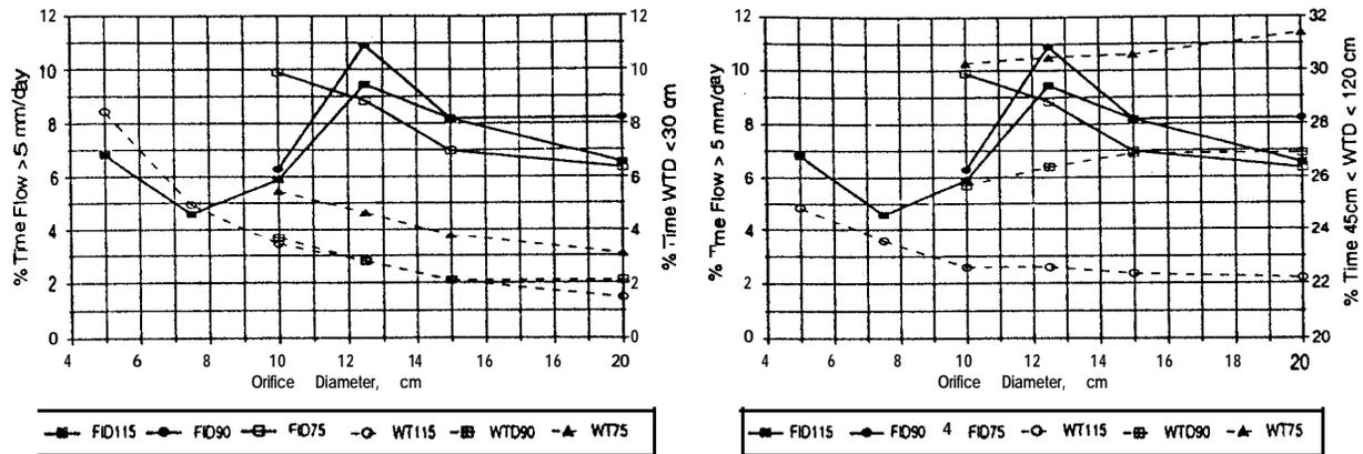
**Fig. 5. Left plot shows percent time flow rates > 5 mm/day and percent time water table within 30 cm depth for different orifice diameters and three depths (75 cm, 90 cm and 115 cm) from the surface. Right plot shows the same but with water table within 45 cm and 120 cm depth. Both the plots shown are for a weir depth of 30cm from the surface.**
