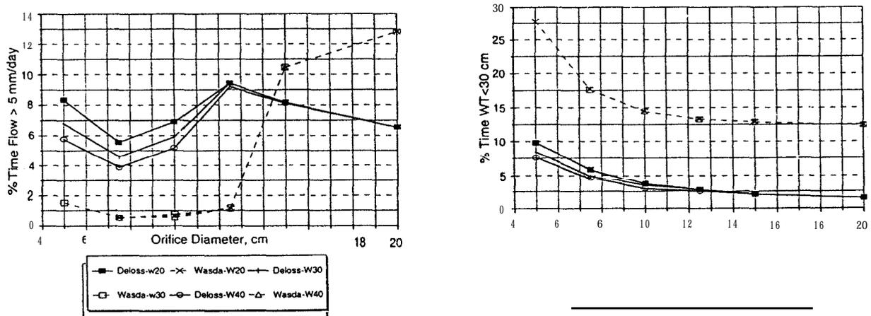
**Fig. 4. Left plot shows percent time flow rates  $> 5$  mm/day for two soils. Right plot shows percent time water table depths were within 30 cm for two soils. Plots shown are for 6 orifice diameters at 115 cm depth and 3 weir depths.**
