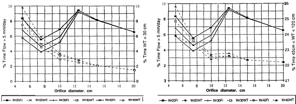
**Fig. 2. Left plot shows percent time flow rates > 5 mm/day and water table depths within 30 cm. Right plot shows percent time flow rates > 5 mm/day and water table depths within 45 to 120 cm during the growing season. Plots shown are for 6 orifice diameters and 3 weir depths with orifices at 115 cm depth.**
