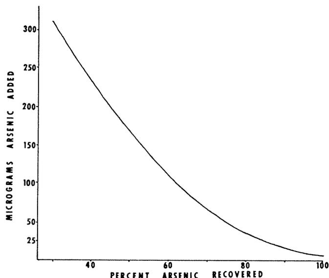
Figure 3. Percent recovery of arsenic as a function of the amount of arsenic added to the arsine generator.
