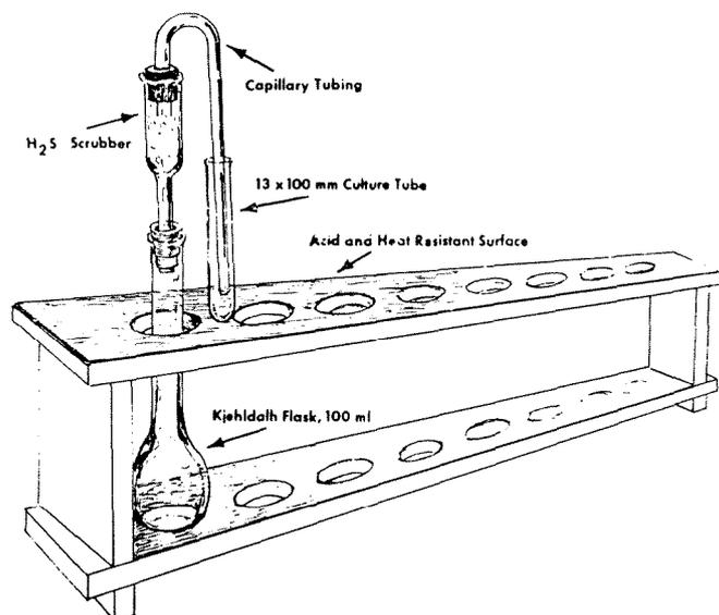
Figure 1. Arsine generator and rack for Kjedahl digestion flasks. Diagram drawn to scale.
