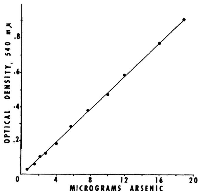
Figure 2. Typical standard curve for arsenic determination as the arsine-AgDDC complex at 540 m $\mu$ . Although the line passes through the origin, the most reproducible readings of optical density are obtained between 0.200 and 0.300 optical density units (4).
