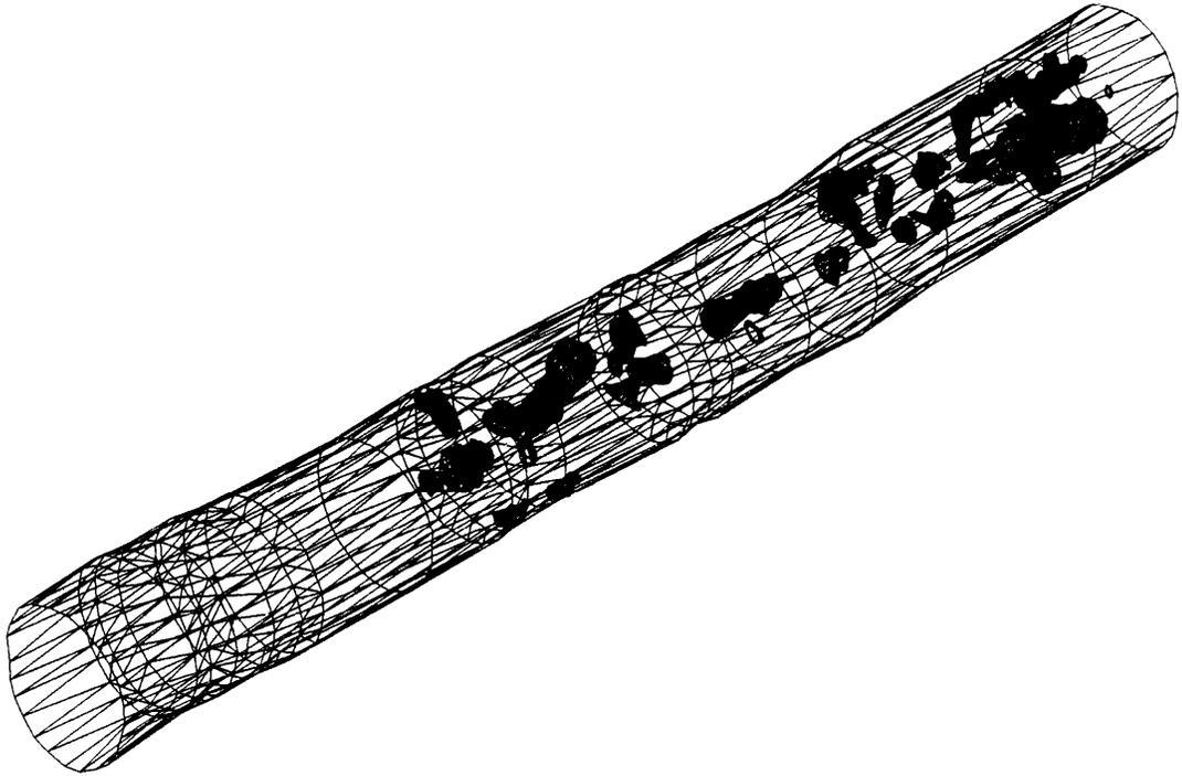
**Figure 3.** Wire frame rendering with internal knot defects revealed.
