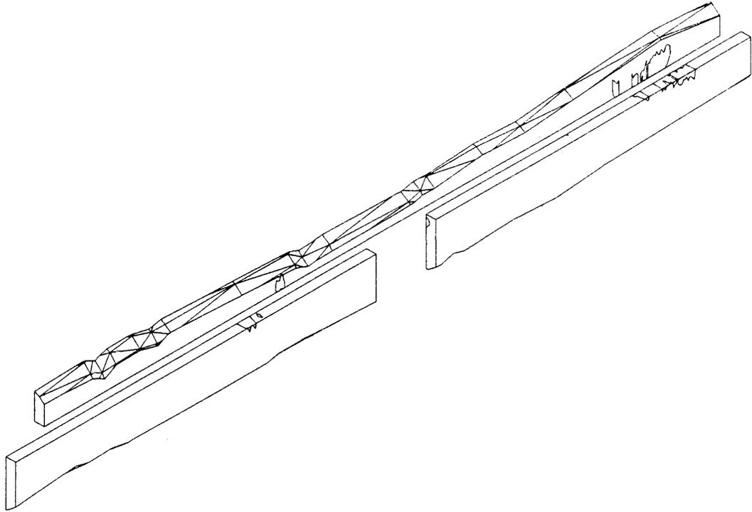
**Figure 7.** Cross-cutting and ripping of flitch.
