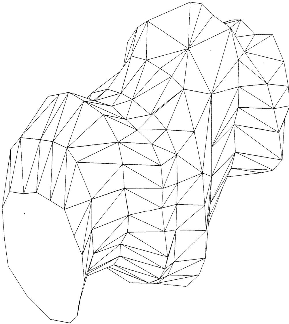
**Figure 2.** Reconstructed knot defect.
