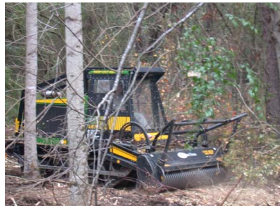
Fig. 1: The GyroTrac GT-25 mulches vegetation in an urban area to reduce the risk of wildfire.
