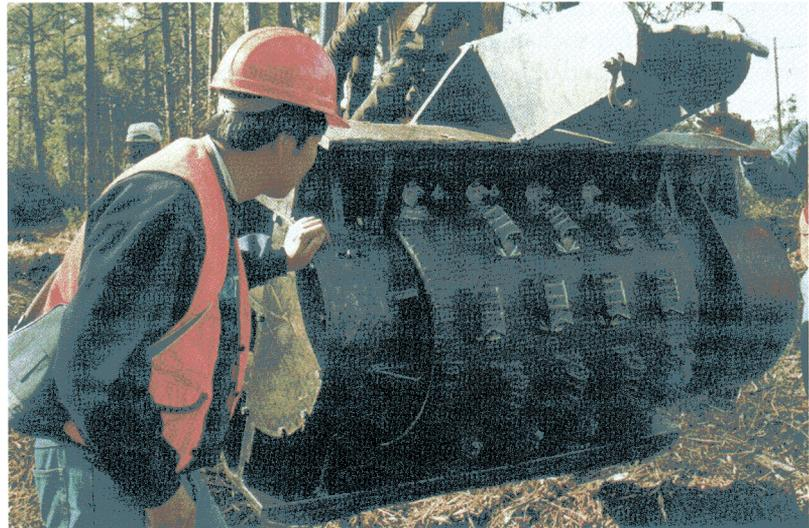
Fig. 1: The Shinn SC-1 boom-mounted rotating drum.
