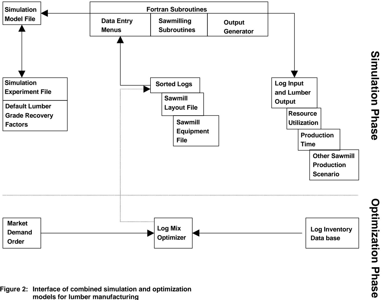
Figure 2: Interface of combined simulation and optimization models for lumber manufacturing
