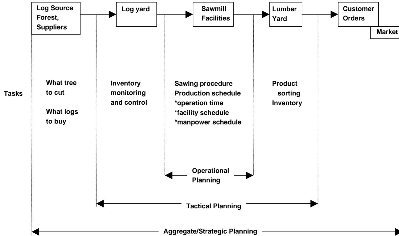
Figure 1: Phases, scope, and tasks in lumber manufacturing
