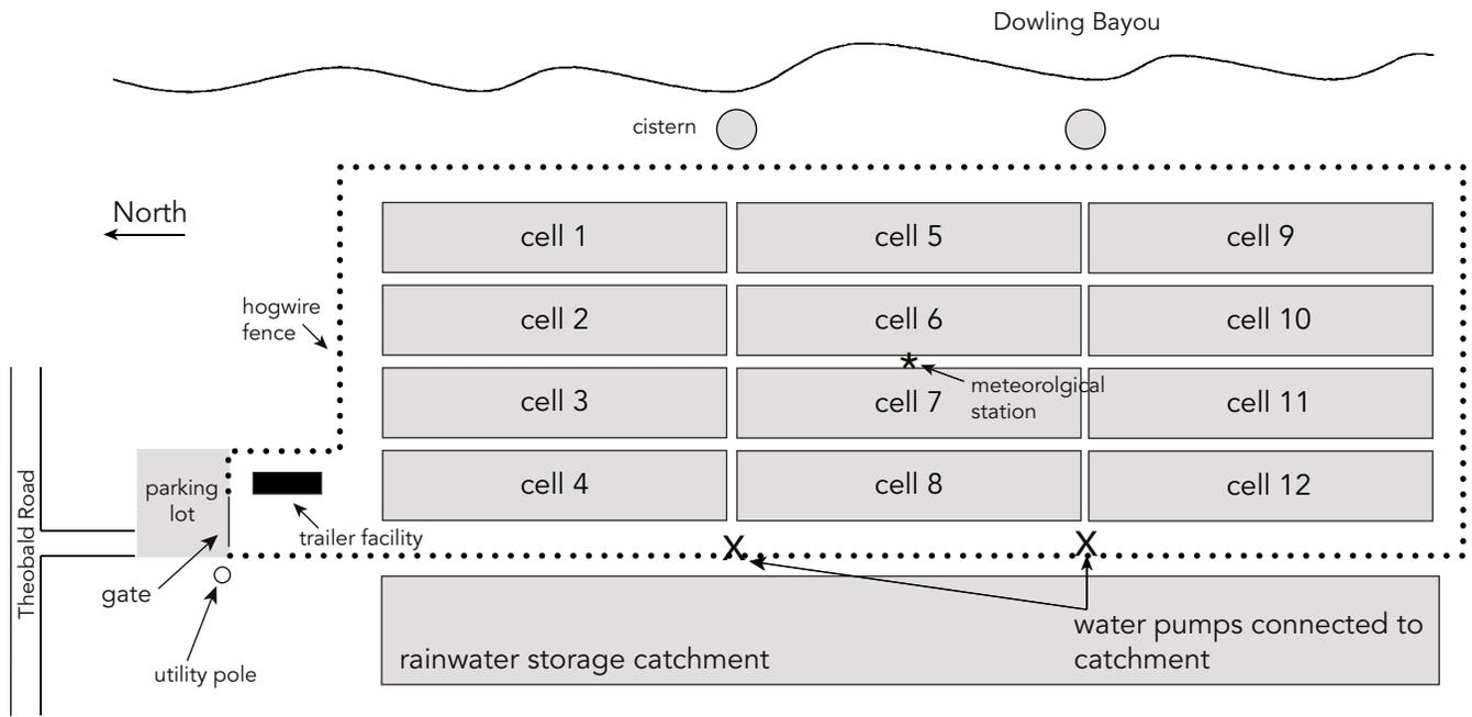
Figure 2. Layout of the Flooding Research Facility including the location of the cells, pumps, and levees.
