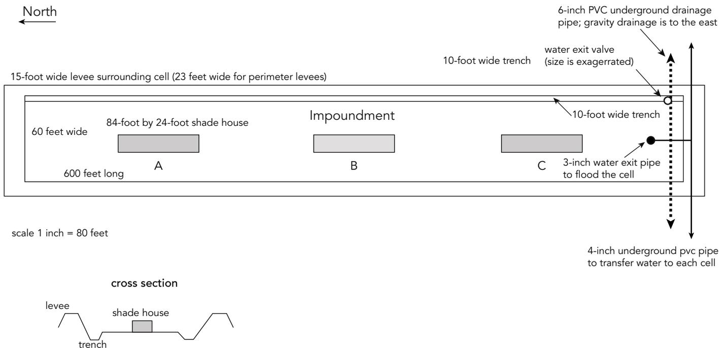
**Figure 4.** Schematic layout of an individual cell at the Flooding Research Facility including shade houses (A, B, C) and the flooding and drainage system.
