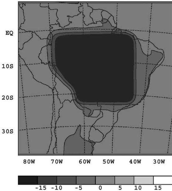
Fig. 5. Direct radiative forcing of smoke ( $\text{W m}^{-2}$ ) without atmospheric feedback simulated with DRM (that is, the difference in the net solar radiation flux at the top model level between the smoke and control simulations).
