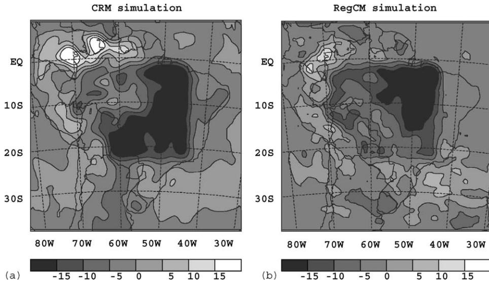
Fig. 11. Direct radiative forcing of smoke ( $\text{W m}^{-2}$ ) with atmospheric feedback. Panel (a) is the difference in the net solar radiation flux at the top model level between the CRM smoke-feedback and control simulations, and panel (b) is the difference between the RegCM smoke and control simulations.
