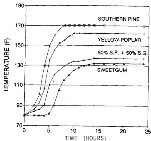
**Figure 1.** Hydration temperature of cement-bonded excelsior boards made from southern pine, yellow poplar, and **sweetgum**
