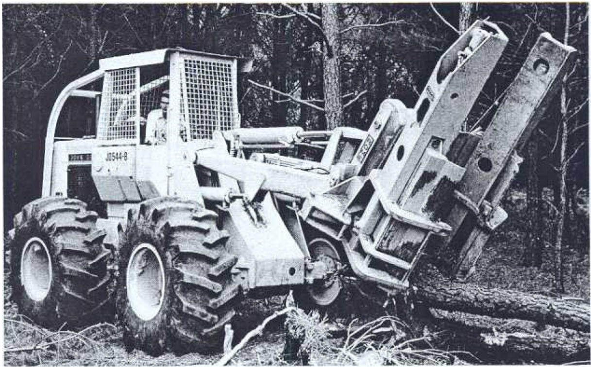
Figure 3. After they are harvested, trees with taproots attached are bunched in conventional fashion to be forwarded by a grapple skidder. Some dirt is loosened as the tree is dropped to the ground.
