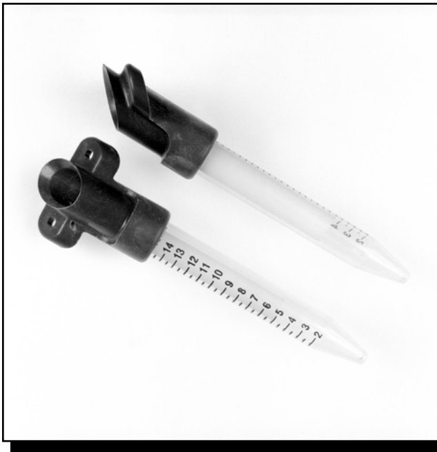
Figure 1—Final sampler design with the fastener holes outside the oleoresin collection area. The sampler directs oleoresin from a wound area on the tree to a plastic 15 milliliter centrifuge tube that screws into the sampler.
