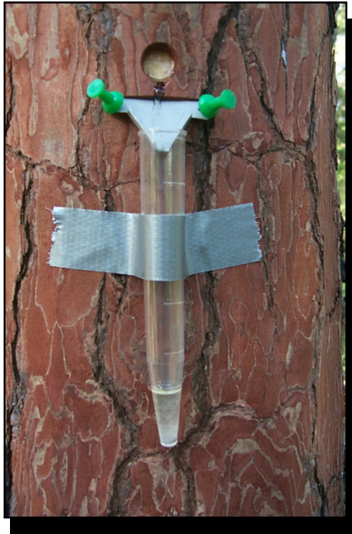
Figure 2—One proposed design used a tin funnel tacked to a tree to direct oleoresin into the collection vial.
