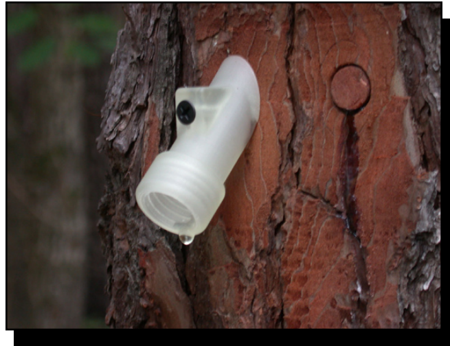
Figure 3—An early design had a single fastener screw in the wound zone. This design was abandoned because the screw was causing more resin to flow than would have flowed otherwise.
