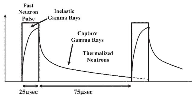
Fig. 2. Pulsing sequence of the neutron generator.
