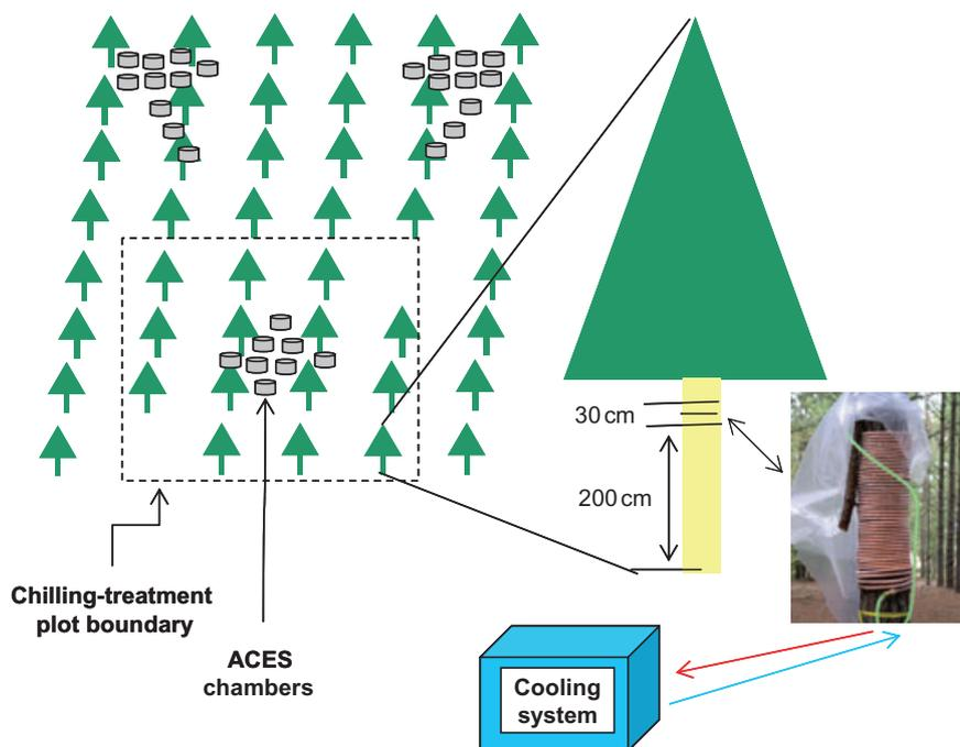
**Figure 1.** Illustration of cold-block installation, including a picture of the stem chilling coil, and the layout of automated carbon efflux system (ACES) chambers used to sample soil CO<sub>2</sub> efflux in the treatment plot and exterior treatment plot (diagram not to scale).
