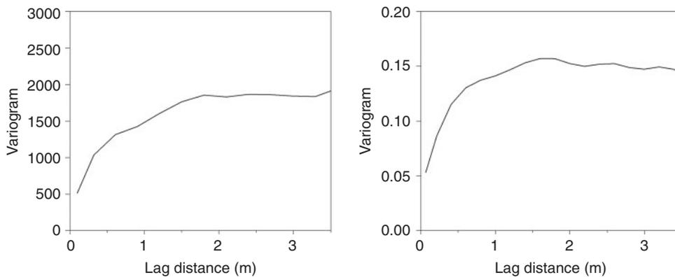
**Fig. 3.** Semivariograms of plot data show that both LIDAR (Light Detection and Ranging) and fire temperatures (90th quantile of temperature readings) both vary at sub-metre scales, as the sill is reached between 0.5 and 0.75 m in both cases.
