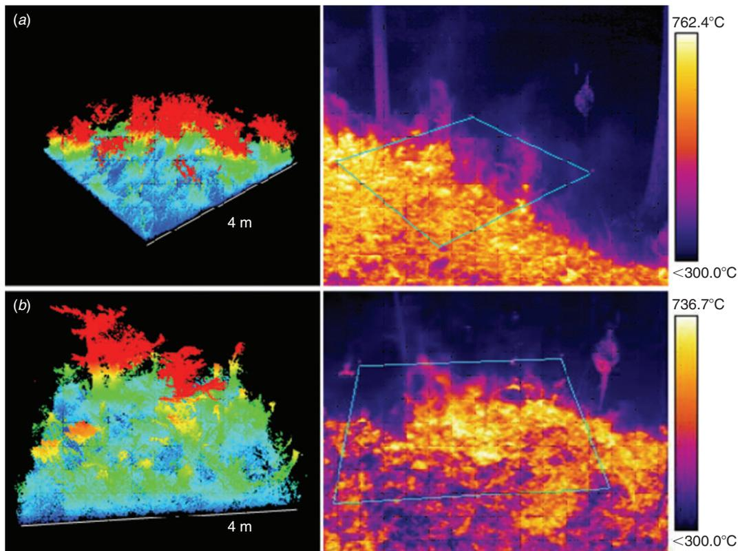
**Fig. 2.** Spatial data to delineate fuel cells required matching (a) LIDAR (Light Detection and Ranging) and (b) *in situ* thermal imagery of burns with georeferenced point intercept data of fuel characteristics.
