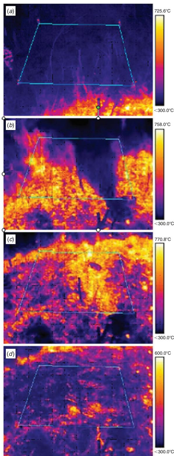
**Fig. 5.** Time series showing the interaction of fine-scale fuel variation and fire behavior in the wake of a pocket gopher mound (Fuel Cell 12: bare mineral soil). Interactions among wildland fuel cells are both critical and complex for predicting fire effects. (a) 23 February 2007 12:17:34; (b) 12:18:31; (c) 12:19:11; and (d) 12:21:42. Total elapsed time was 4 min 8 s.
