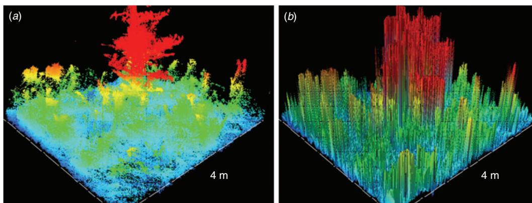
**Fig. 1.** Ground-based LIDAR (Light Detection and Ranging) image of  $4 \times 4$  m plots: (a) sub-cm density point cloud illustrating the accuracy of this tool; and (b) Triangular Irregular Network (TIN) of LIDAR data used in spatial analysis and mapping of fuel bed heights.
