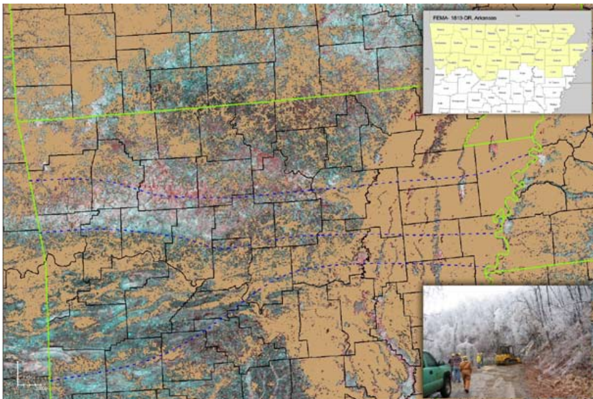
Figure 5. View of forest damage from a major ice storm across northern Arkansas, USA, January 26–28, 2009. RGB composite image was made by loading the maximum 2009 NDVI for June 10–July 15 in the blue and green, and loading the maximum 2001–2006 NDVI for June 10–July 27 into red. Areas with drops in maximum NDVI are shown in red tones, and correspond well to dotted blue ice accumulation isopleths (1-2+ in, 0.5-1 in, and 0.25-0.5 in from north to south, respectively) and Federal Emergency Management Agency declared disaster counties shown in the upper right inset. This was the worst icing since December 2000, leaving 350,000 residents without power and causing 18 fatalities.
