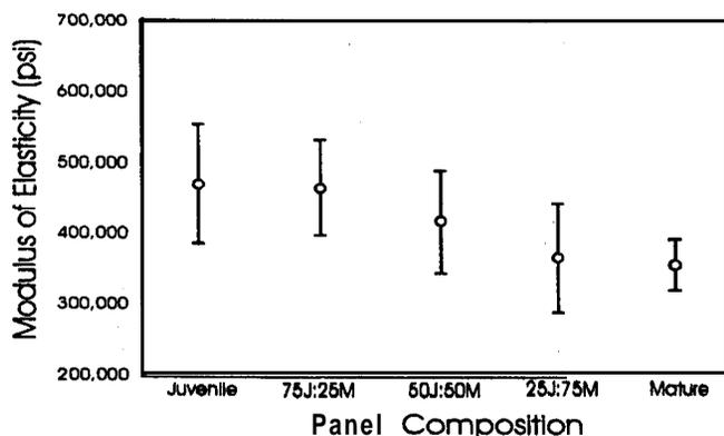
**Figure 1.**— Full-sized MDF panel MOE shown as a function of juvenile: mature wood ratios. Vertical bars represent one standard deviation.
