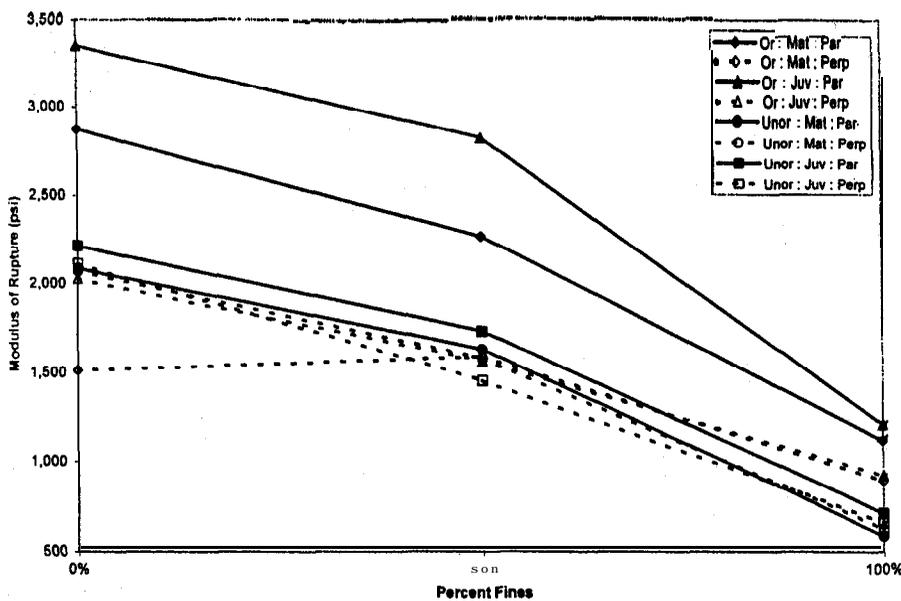
Figure 5.-Effect of fines loading on the MOR of oriented and un-oriented MDF mini-panels.
