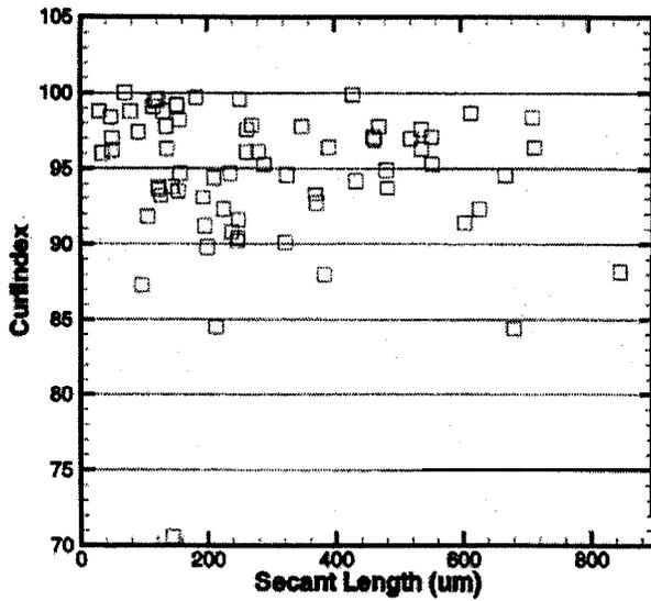
Figure 14.-Fiber curl index vs. fiber secant length of 71 fibers from interior of MDF specimen.
