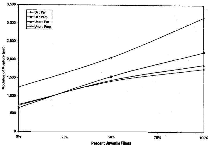
Figure 4.—MOR of un-oriented and oriented MDF mini-panels in relation to percent of juvenile fiber content.
