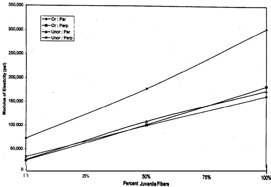
Figure 3.—MOE of un-oriented and oriented MDF mini-panels in relation to percent of juvenile fiber content.
