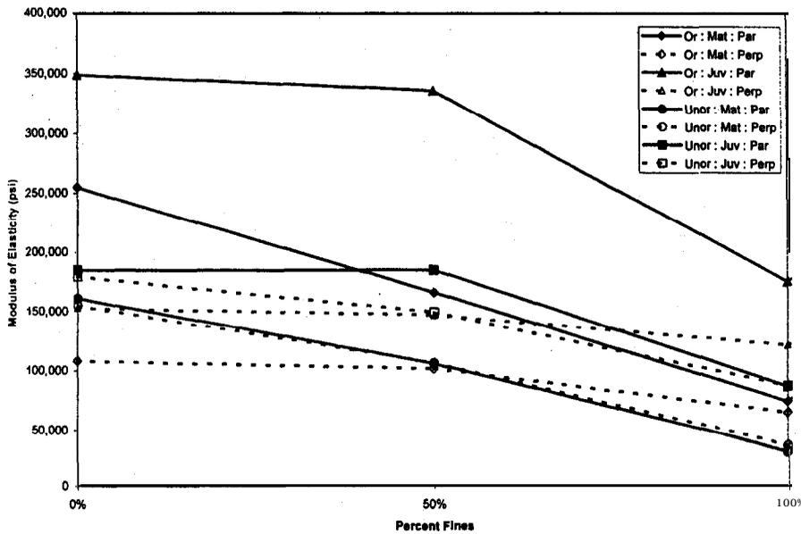
Figure 1.-Effect of fines loading on the MOE of oriented and un-oriented MDF mini-panels.
