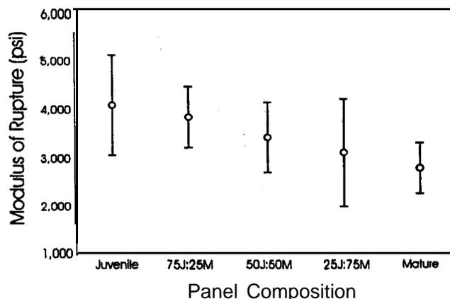
**Figure 2.**- Full-sized MDF panel MOR shown as a function of juvenile: mature wood ratios. Vertical bars represent one standard deviation.
