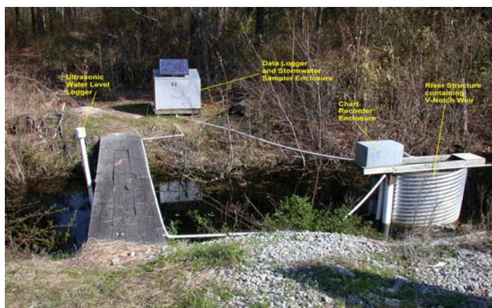
Figure 2. Typical outlet station setup with data logger enclosure, chart recorder, riser structure containing V-Notch weir, and backup ultrasonic water level logger.
