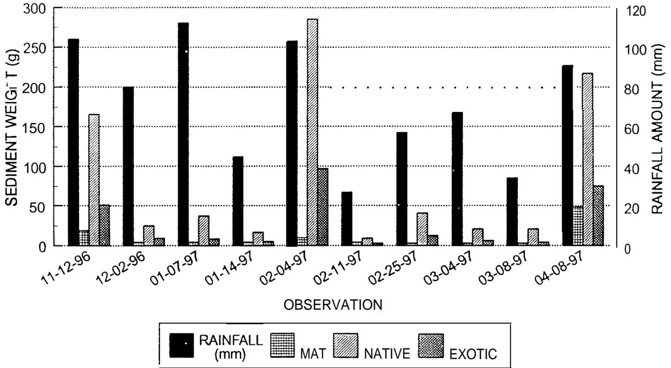
Figure 2. Fillslope Sediment Production -- Mitigation Treatments (1997).
