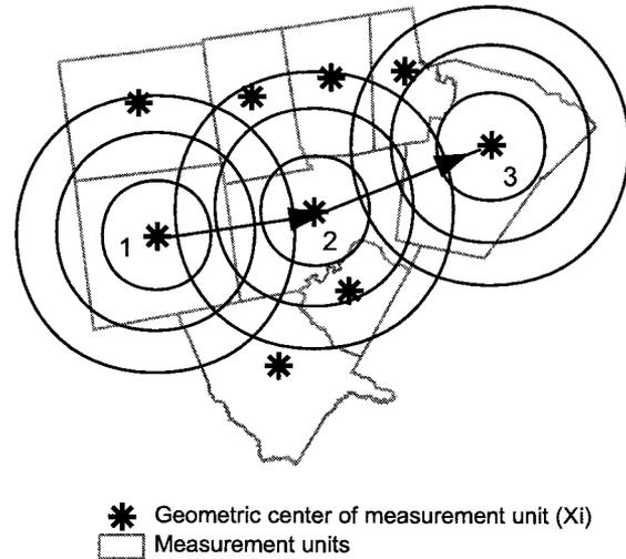
**Figure 1.** Hypothetical example of the scanning process. In this example, the scanning procedure starts at measurement unit 1 where a set of concentric circles are generated and  $\Psi_w$  is calculated for each circle around measurement unit 1. Once the maximum circle size is achieved (say 20% of the area), then the procedure is then carried out at measurement unit 2. This process is carried out for each measurement unit.
