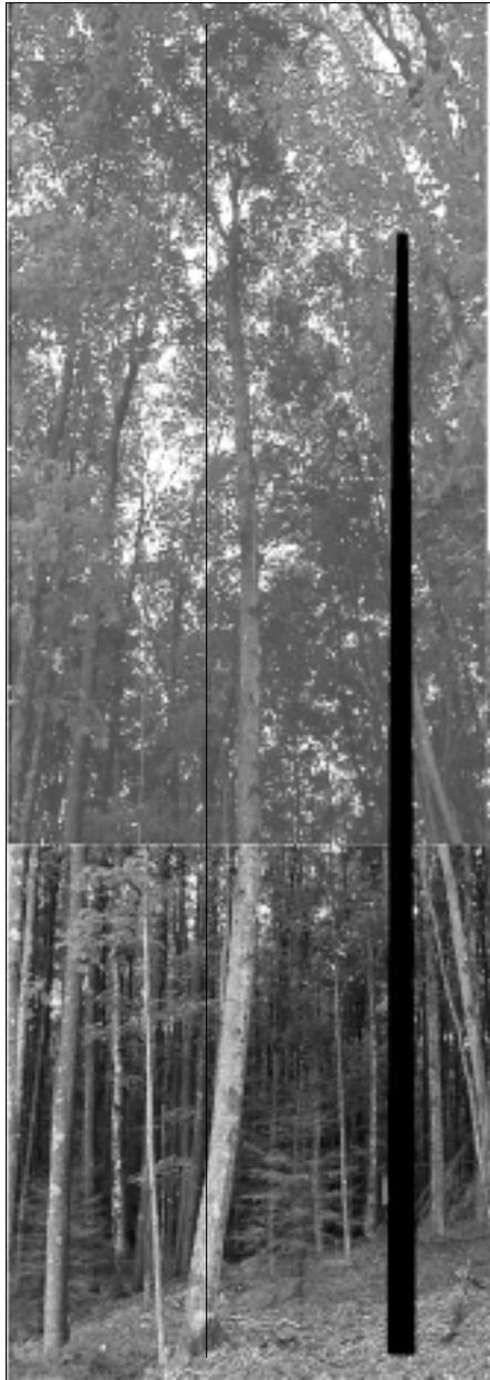
Figure 4. Overlapped images of stem showing offset between datum plane and the actual stem axis. black silhouette represents information derived from a volume model assuming correct taper function is used.
