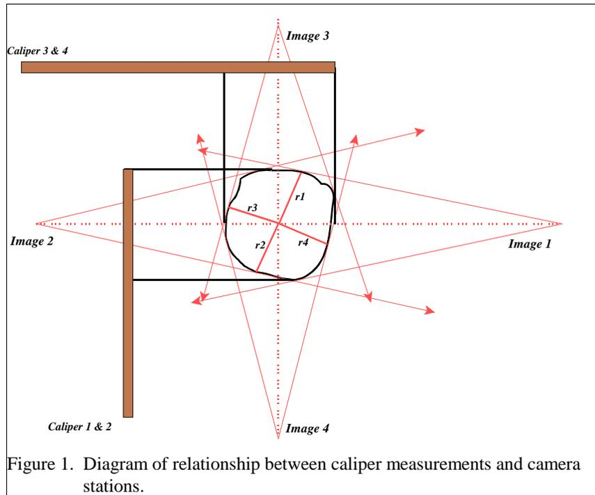
Figure 1. Diagram of relationship between caliper measurements and camera stations.
