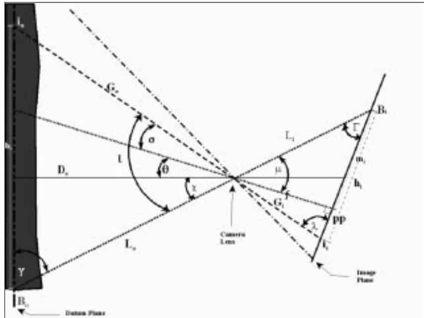
Figure 2. Identification of the variables used in the calculations. Angles are indicated by Greek letters corresponding to the variable name of their opposite side. The subscripts **o** and **i** reference object and image space measurements, respectively.
