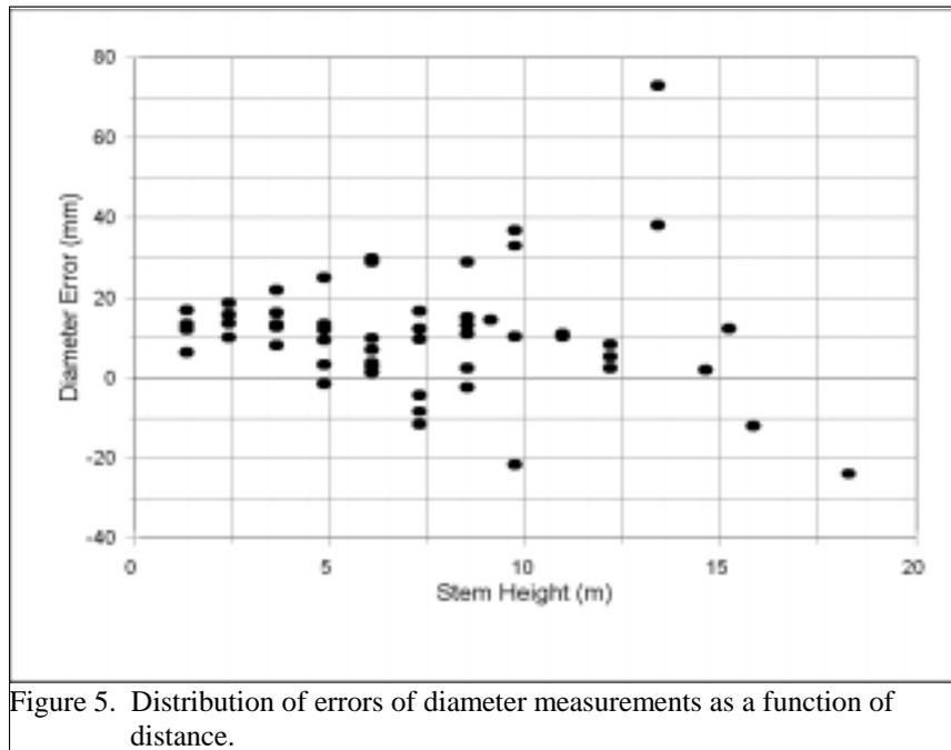
Figure 5. Distribution of errors of diameter measurements as a function of distance.
