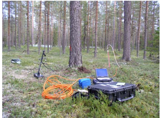
Figure 1. GSSI Sir-20 radar unit, 900 MHz antenna (left) and TubeWave-1000 (right) on opposite sides of Scots pine tree.
