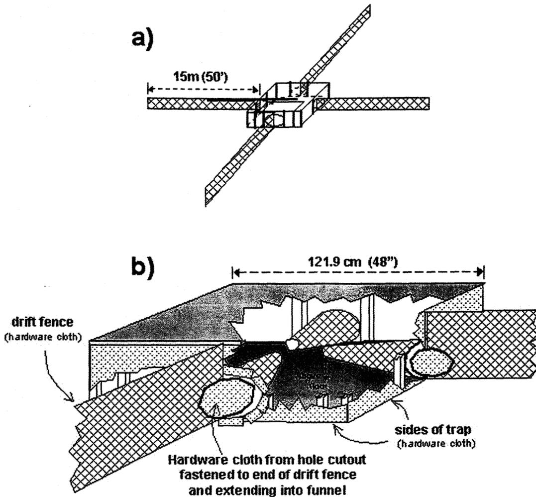
**Cut-away view of drift fence attachment and placement**
