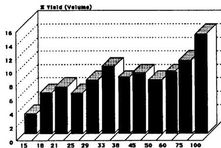
Figure 2. An example tally sheet and the companion graph of cutting lengths for computer analyzed lumber illustrates the type of information that can easily be provided for each package of lumber using an automated system.
