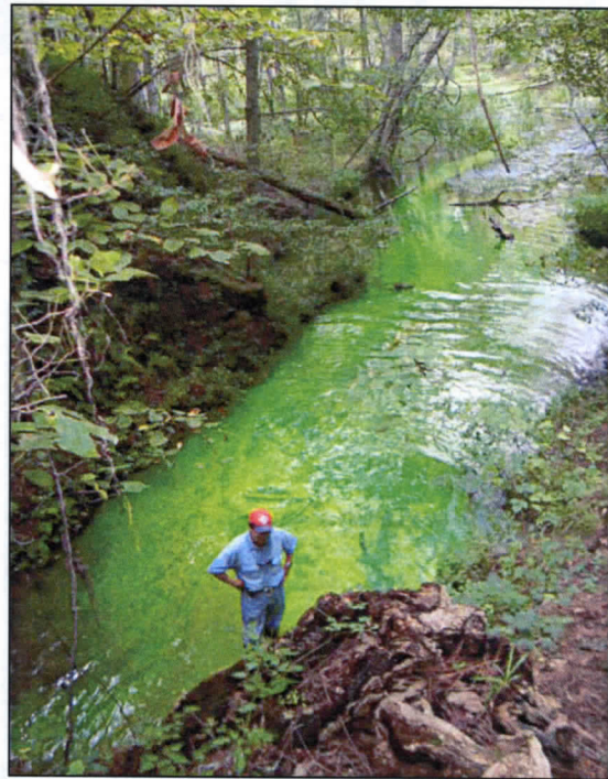
Dye trace conducted in September 2008 to determine flow paths and times to the cave spring at the CBC headwaters. Picture is at the cave spring. Image: A. Edwards
