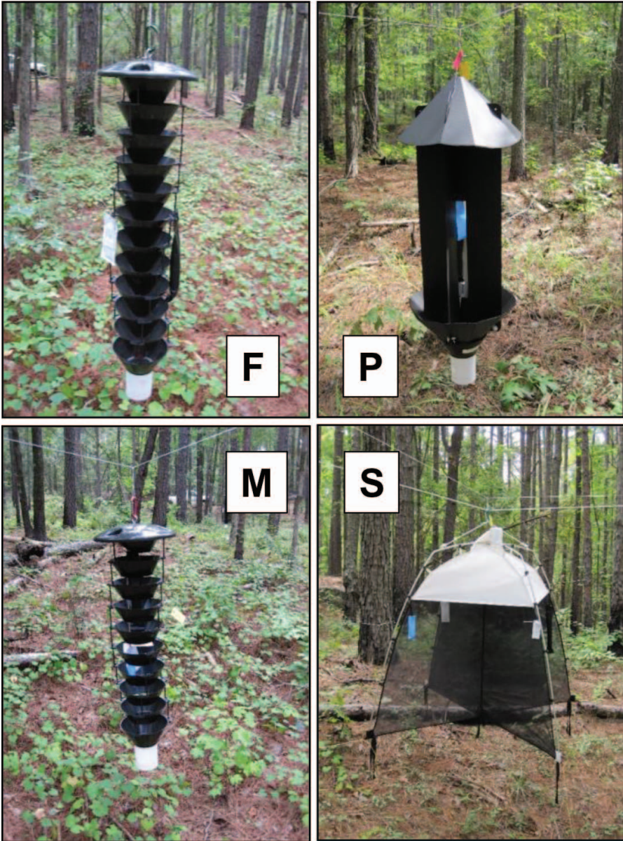
Fig. 1. Trap types used in northcentral Georgia (13 September–25 October 2012): 12-unit standard multiple-funnel trap (F); panel trap (P); 10-unit modified multiple-funnel trap (M); and sea, land, and air Malaise trap (SLAM [S]). All traps were baited with black ethanol, blue \alpha -pinene, white ipsenol, and white ipsdienol lures.
