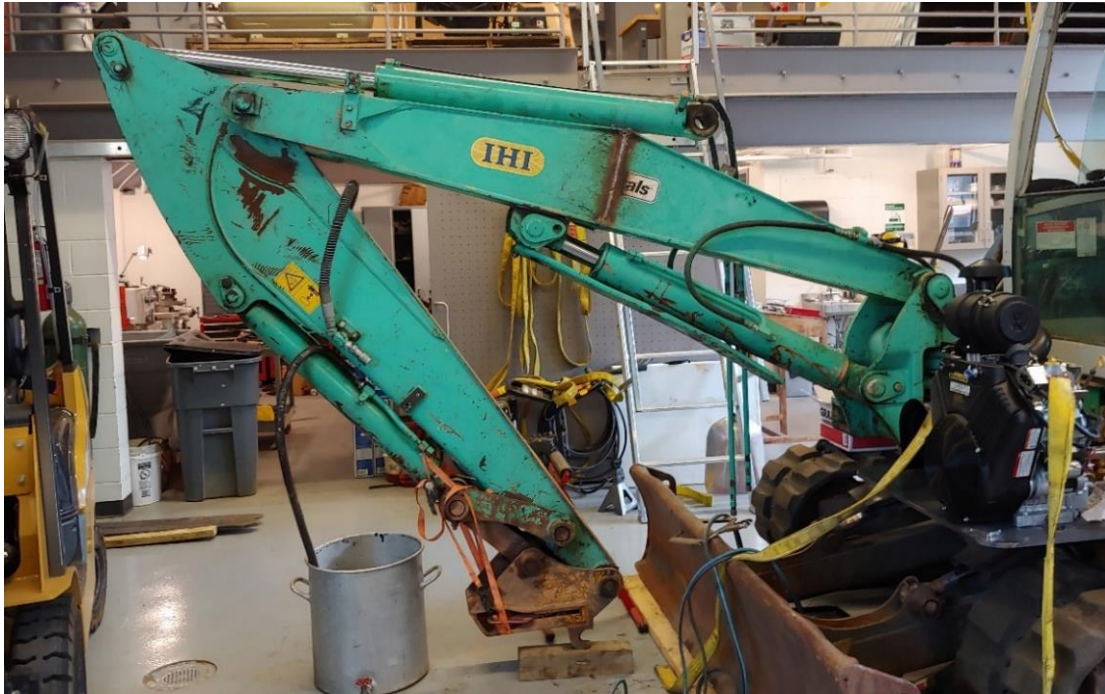
Figure 1: Small excavator with modified boom
