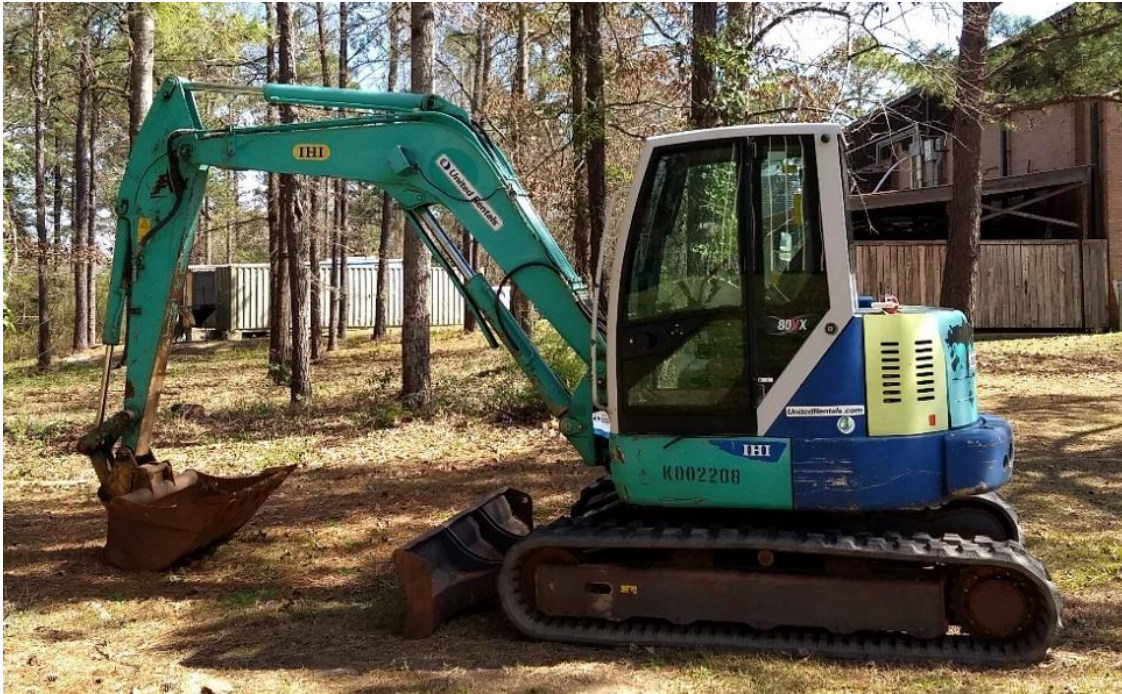
Figure 1: Small excavator (IHI 80VX)
