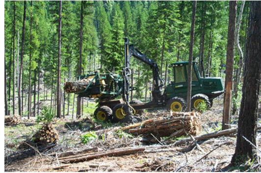
Costs of Mechanical Fuel Reduction Treatments, Fig. 2 Bundler creating composite logs near Idaho City, Idaho, USA
