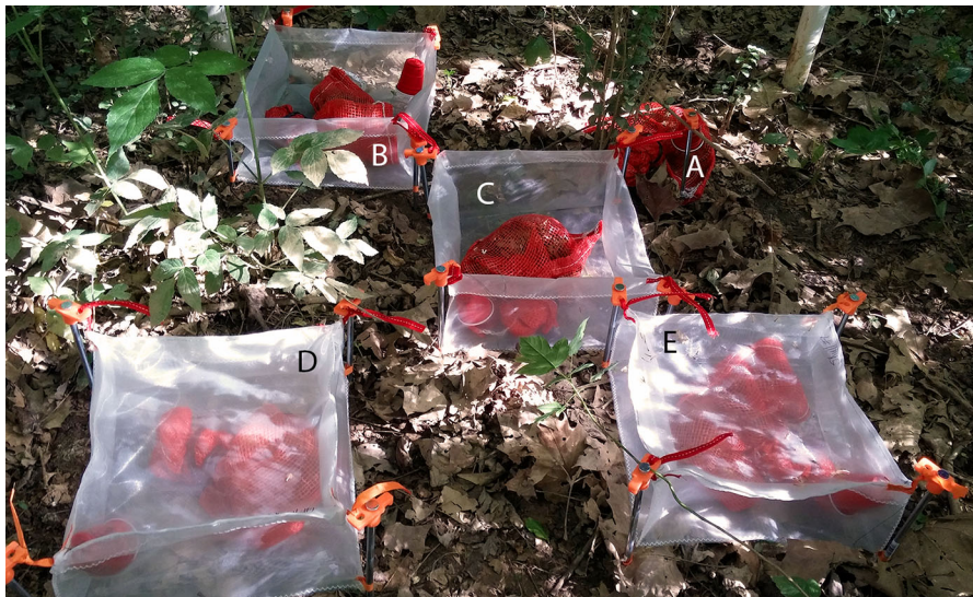
Fig. 1 Example of litter basket treatments. Letters denote treatments as follows: a no basket, b open-top, c open-top with slits, d closed-top, and e closed-top with slits
