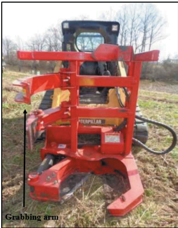
Figure 2. Fecon shear head with opened grabbing arm.
