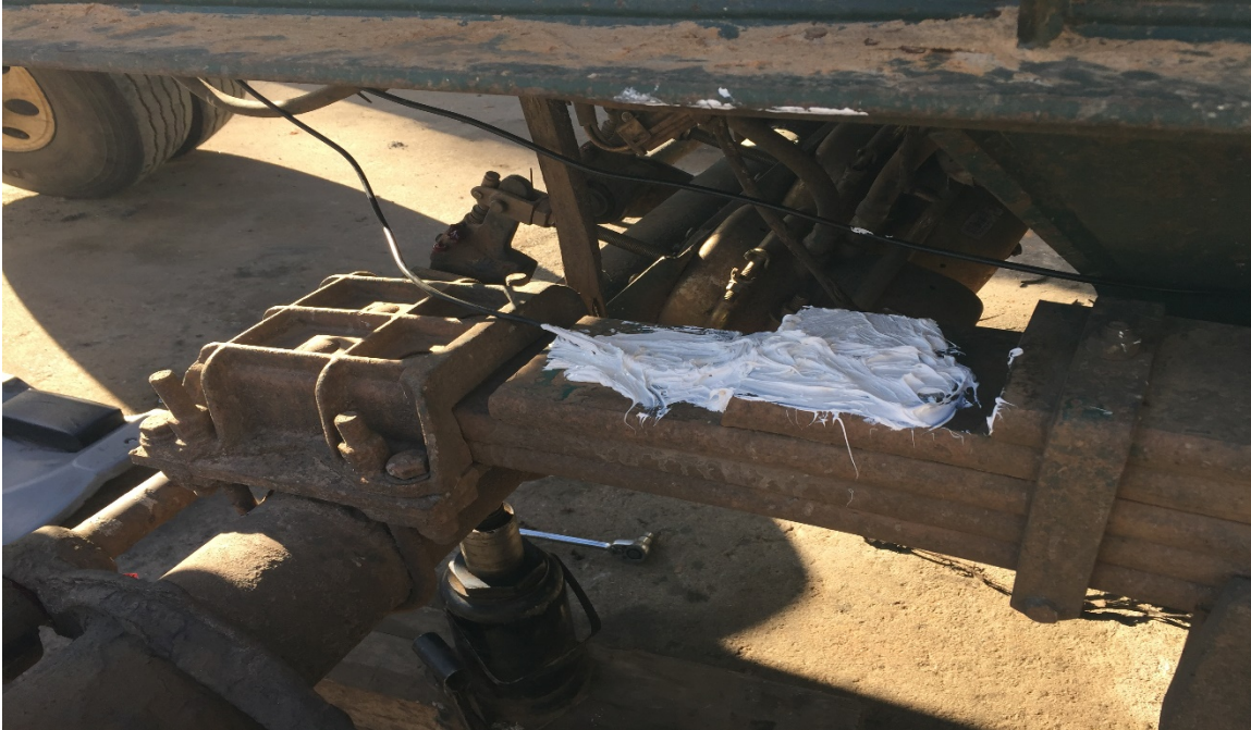
Figure 3: Strain gauge coated in protective caulk.
