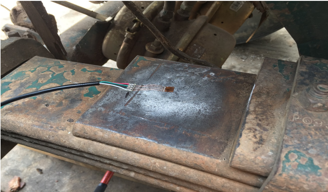
Figure 2: Strain gauge adhered to leaf spring.
