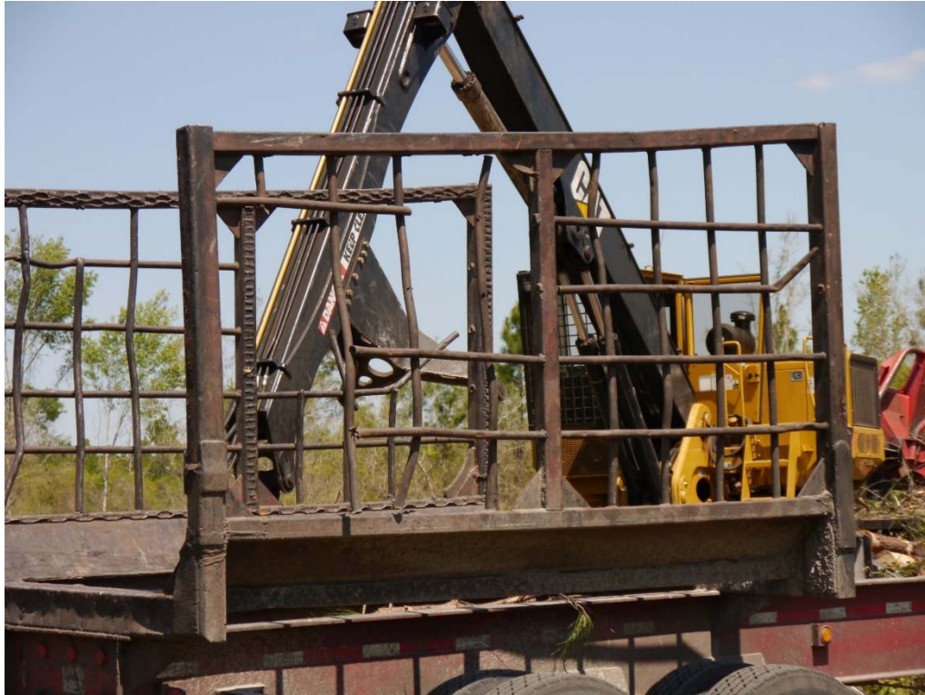
Figure 2: Log trailer with "basket" for hauling untrimmed trees.
