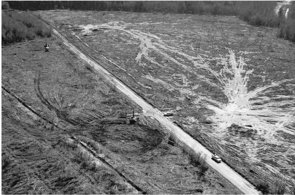
Fig. 8.1. Picture of soil conditions after harvesting on a plantation pine site, contrasting subsurface drainage (left of the road) with that without improved drainage (right of the road). Note severe puddling of soil in contrast with soil conditions on left of the road, where drainage had been improved. (Photo by Joe Hughes, 1981.)
