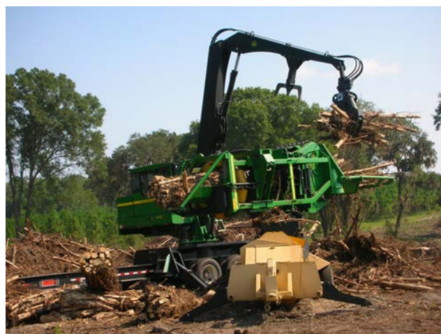
Fig. 4 A John Deere slash bundler. Photo: Mitchell
