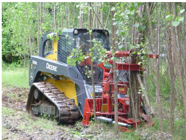
Fig. 5 A John Deere skidsteer mounted with a shear feller head attachment for harvest and tending in coppice systems. Photo: Mitchell
