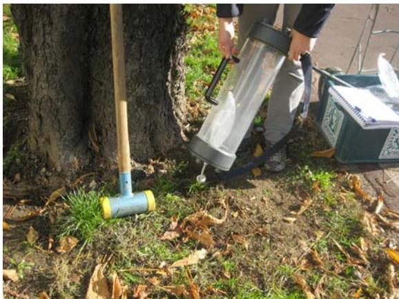
**Fig. 4.** The automatic pump employed in the field to put directly soil air in Nalophan bags.
