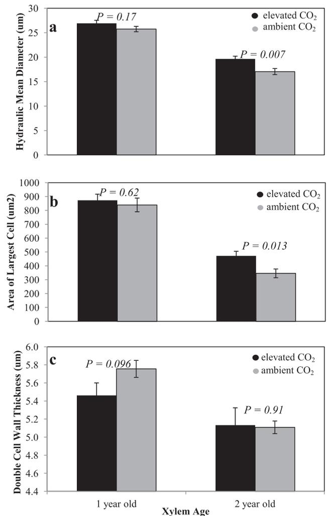
**Fig. 2.** The hydraulic mean diameter (a), the area of largest cell (b), and double cell wall thickness of elevated and ambient CO<sub>2</sub> treated branch tissue of sweetgum. Significance level ( $p < 0.05$ ) among control and CO<sub>2</sub> enriched samples are shown based on 2 sided t-test.
