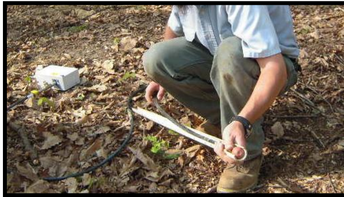
Figure 4. Visual of hydraulic hose, bulb, and box used to house electronic components.
