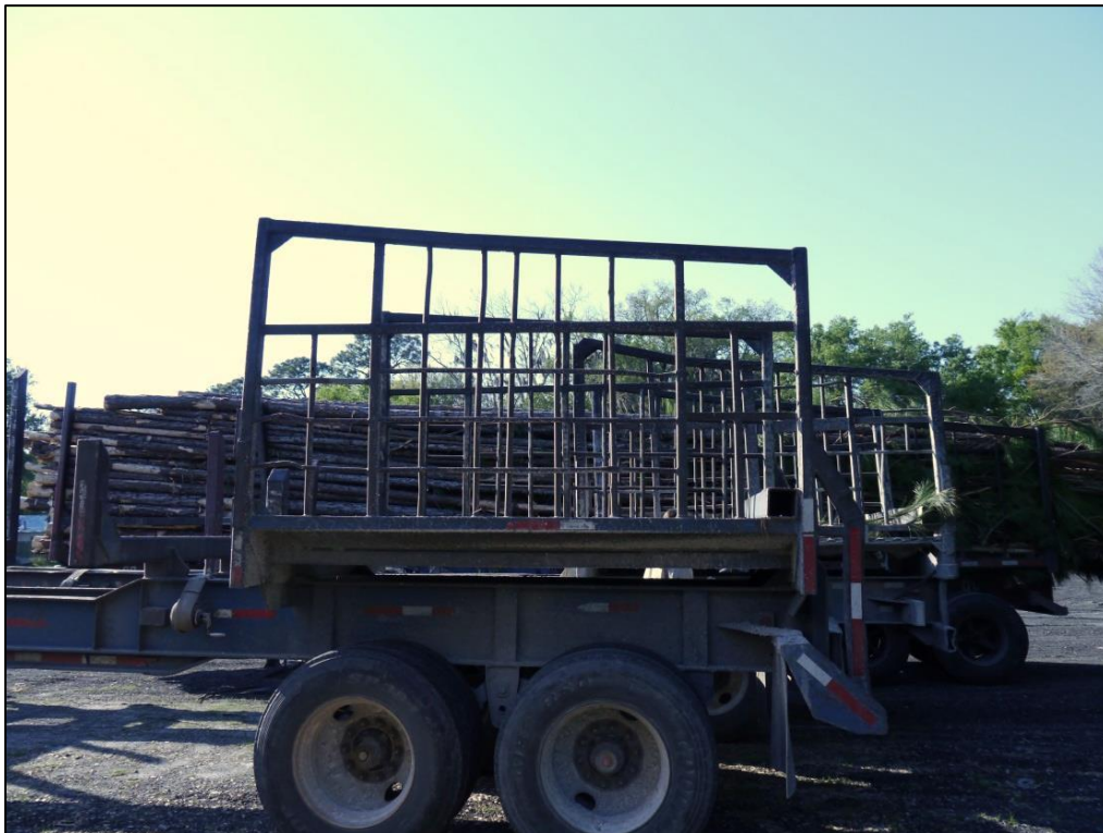
Figure 4: A logging trailer with a raised belly pan in the rear "basket".
