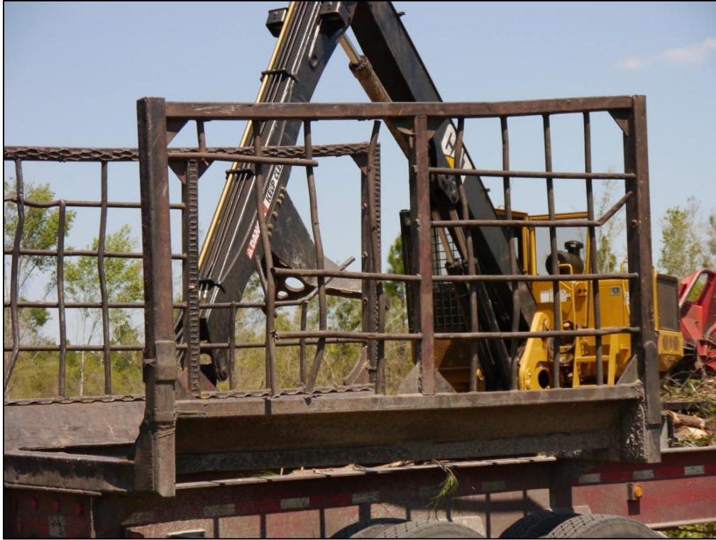
Figure 1: A logging trailer modified with a “basket” for hauling untrimmed pulpwood.
