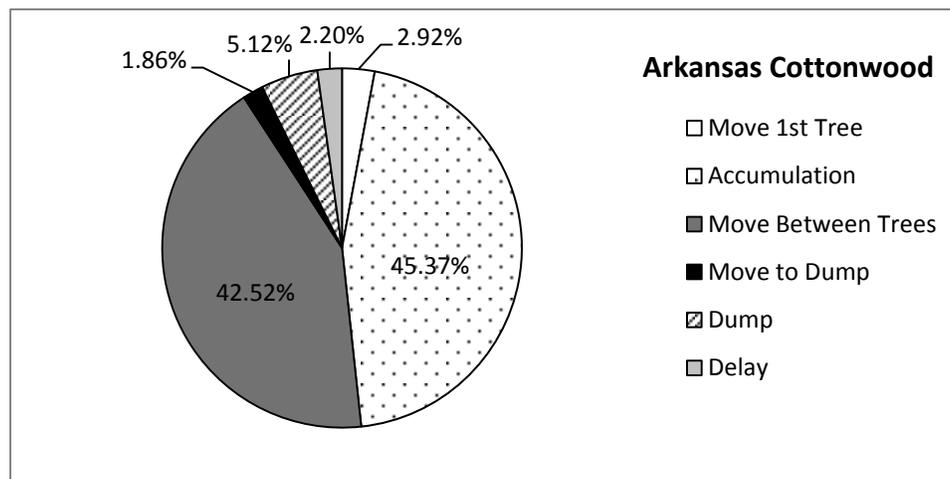
Figure 3. Elemental Cycle Time (%) for Stand 3
