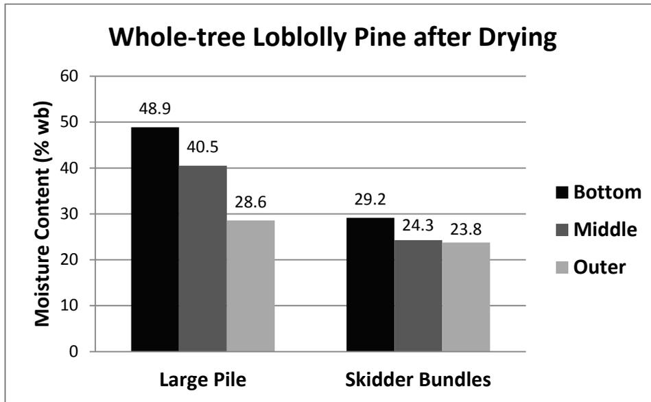
Figure 3. Comparison of moisture content among zones within each pile type.
