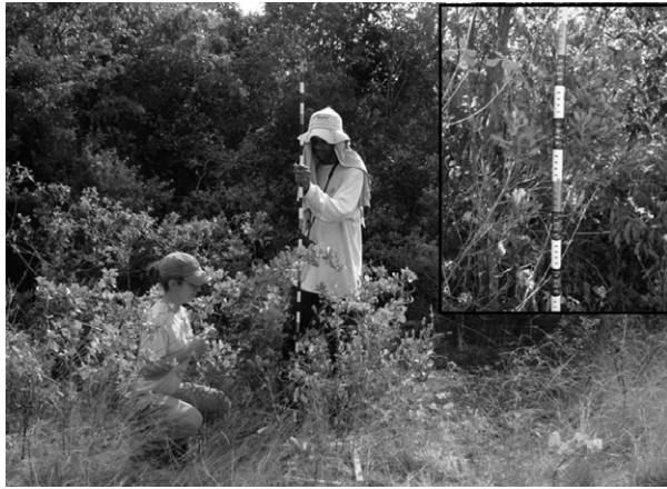
Fig. 1. Apparatus and procedure used for visual obstruction estimation, demonstrated in a low-biomass quadrat, with the inset showing details of the PVC pole. Each coloured band on the pole is 5-cm wide. Grey bands designate the upper limit of each 25-cm vertical height class.
