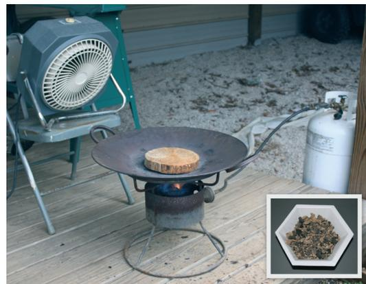
**Fig. 1.** Set-up for burning wood to isolate soil carried in by termites. A resulting soil sample is shown in the inset.
