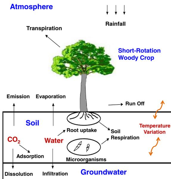
**Fig. 1** A schematic diagram showing the mechanisms of CO<sub>2</sub> emission from a short-rotation woody crop plantation as affected by soil water and temperature regimes as well as by surficial processes
