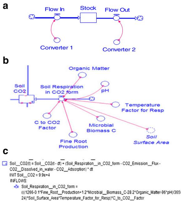
**Fig. 2** A schematic diagram showing the four key features of STELLA (A) (1) stock, (2) flow, (3) converter, and (4) connector and the example translation of soil respiration processes into STELLA model (B) associated equations (C) that were generated automatically by STELLA
